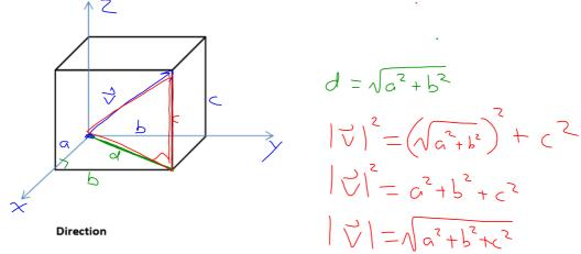
The direction of a vector in 3-space is described by finding the measure of the angles it makes with the **positive** x, y and z axes. These angles are named  $\alpha$  (alpha),  $\beta$  (beta) and  $\gamma$  (gamma) respectively. These angles always form a right triangle with the vector being the hypotenuse and with the respective coordinate axis being the adjacent side.
