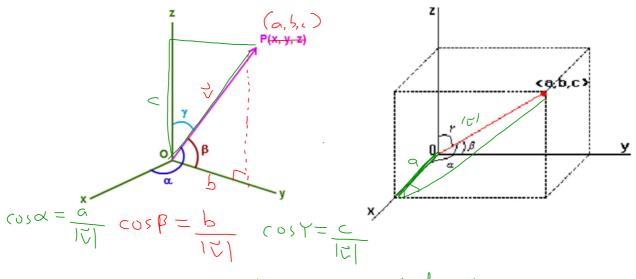
cos &, cos B, cos T are called direction cosines. X, B and Y are direction angles. A special relationship exists between the direction cosines.
