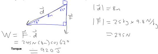
A force that causes an object to turn is called torque. (Consider using a wrench).
